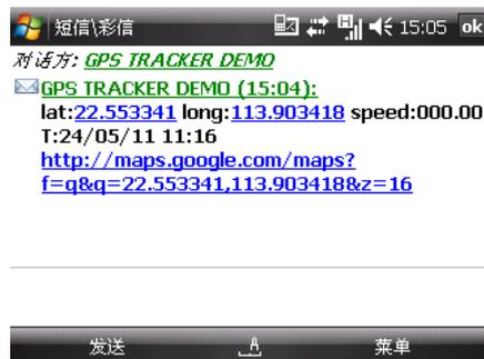
\*When lost fix to satellites, it will track by LBS / CELL-ID. And the SMS will include two positions:
